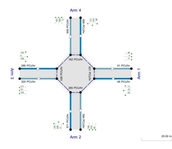
Showing modelled flow through junction (PCUftr). Time Segment: (11:00-11:15) Showing Analysis Set "A1 "; Demand Set "D2 - Survey, Sat "
